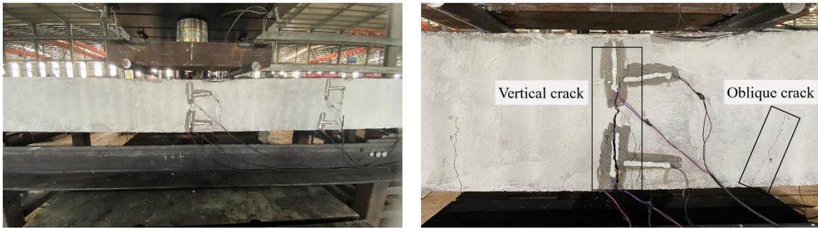
**Figure 7.** Failure characteristics of the BEJC50 × 6 component.
