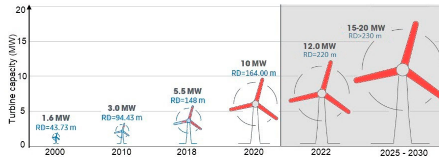
Figure 4. Power and rotor diameters of existing and planned offshore wind farms [2].
