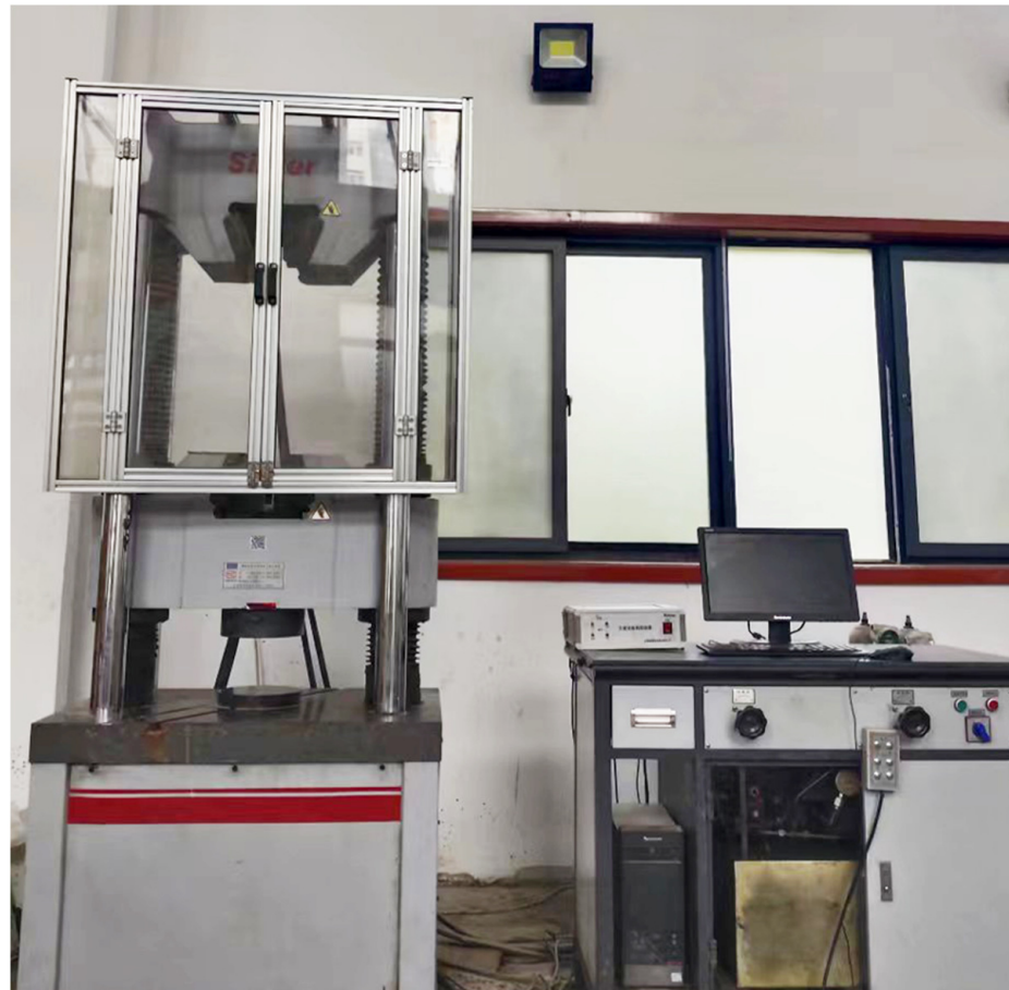
Figure 1. The WAW-1000D microcomputer-controlled electro-hydraulic servo universal testing machine.
