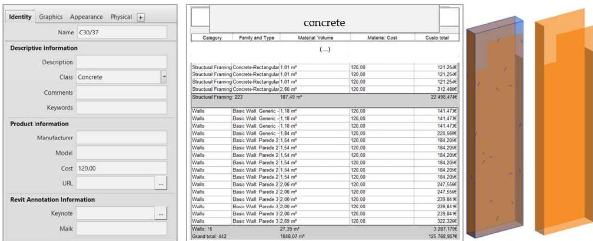
Figure 18. Quantity take-off of concrete and the formwork of a column.
