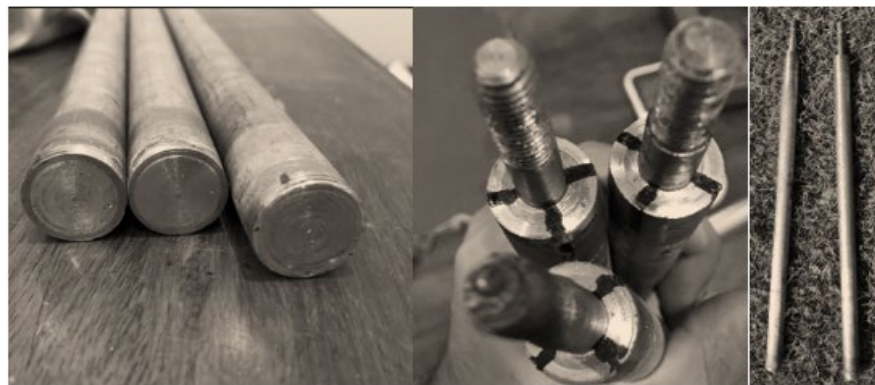
Figure 3. Galvanized iron pipes used as a pile in model piled raft.
