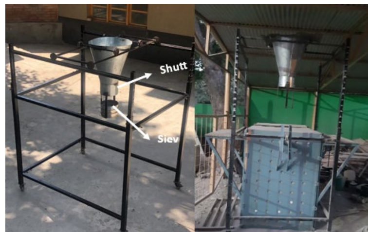
Figure 5. Mobile pluviator installed above the soil box.
