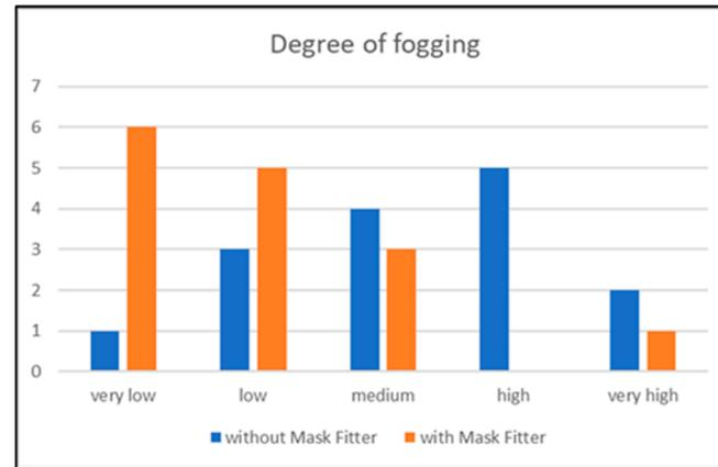
**Figure 11.** Effects of Mask Fitter on fogging of loupes and glasses.
