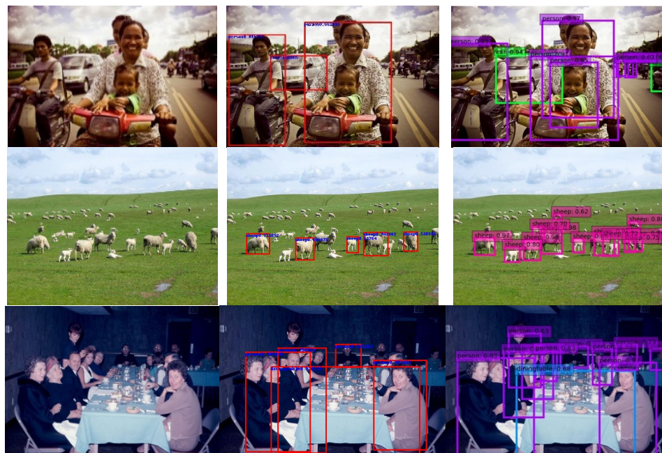
Figure 9. Detection examples comparison of the conventional SSD and our proposed algorithm on the PASCAL VOC 2007 test. For each group, the left side is the original image, the middle is the detection result of SSD and the right side is the detection result of our algorithm.
