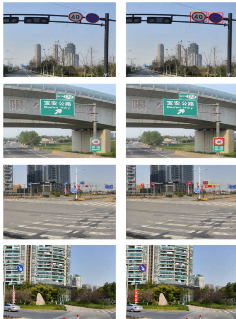
Figure 13. Images demonstrating the effect of improved Faster R-CNN detection (images on the left are the original images, and those on the right are the detection images).
