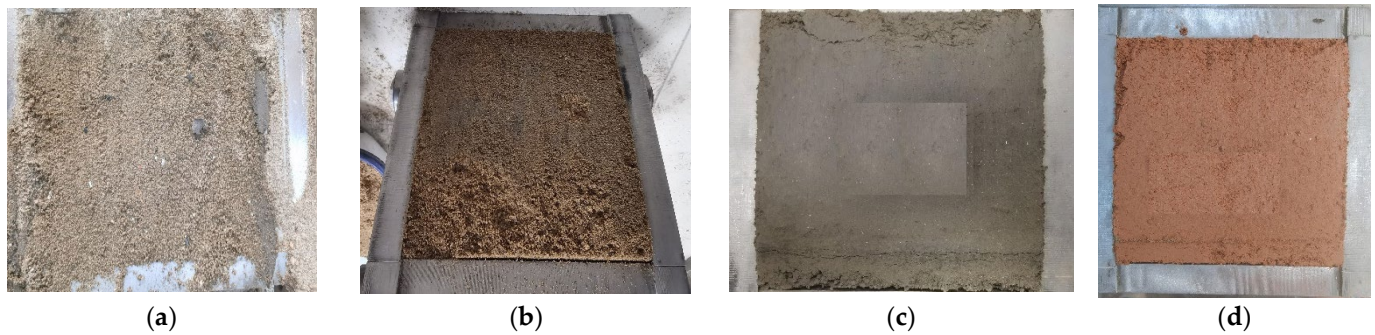
Figure 5. Examples of interface shear surfaces: (a) silty sand, (b) medium-coarse sand, (c) clay, and (d) sandstone.
