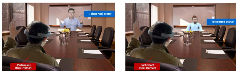
Figure 1. 3D MR tele-conference system to collaborate at a local site with a teleported avatar of the remote participant. The MR tele-conference system can make various typed teleported avatars; for example, a realistic avatar capturing the remote participant ( left ), and a pre-built character-like avatar using a 3D modeling toolkit ( right ).
