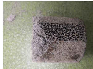
Figure 13. Surface speckle pattern of specimen.
