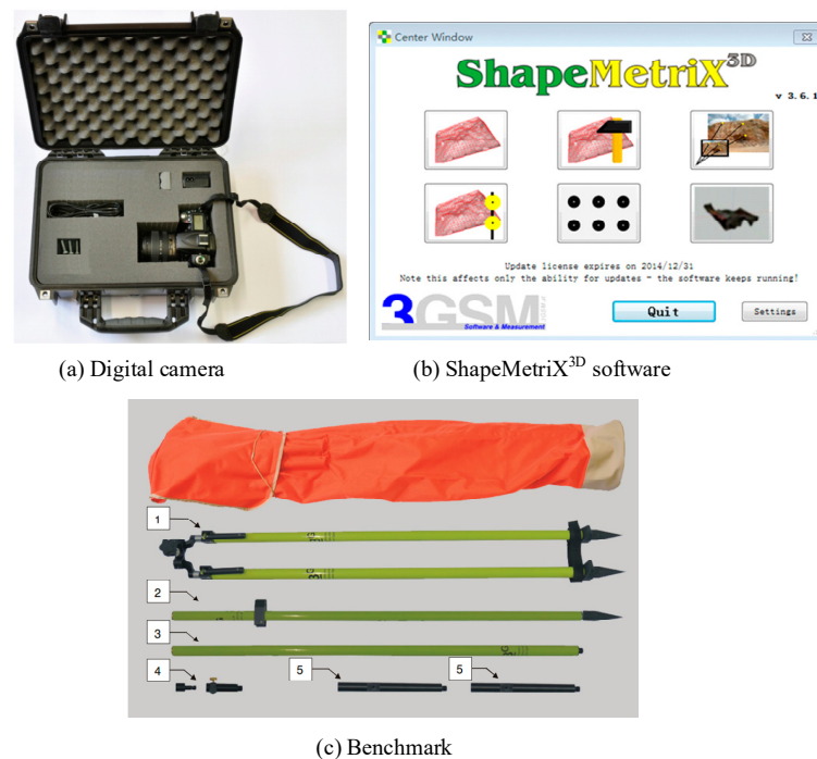
Figure 2. Composition and principle of the ShapeMetriX 3D system. Research steps 1–5 are the process of data collection based on the equipment.
