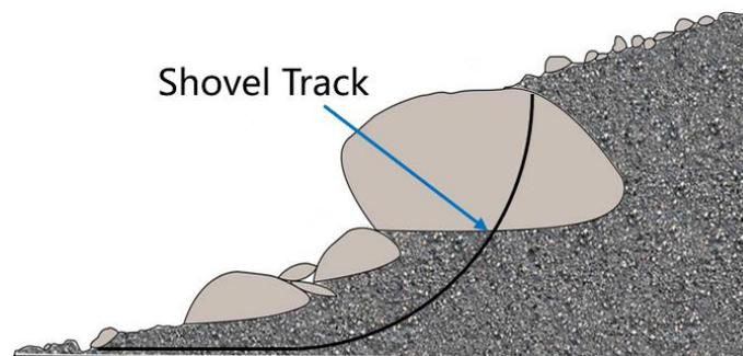
**Figure 8.** Example for improper shoveling trajectory planning [47].
