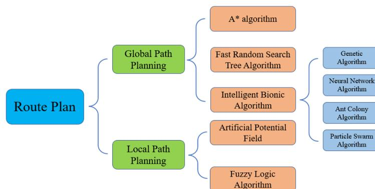
Figure 9. Path planning methods for underground intelligent LHD [12,85,86].
