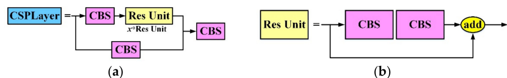
Figure A1. The structure diagram of CSPLayer and Res Unit: (a) CSPLayer structure (b) Res Unit.
