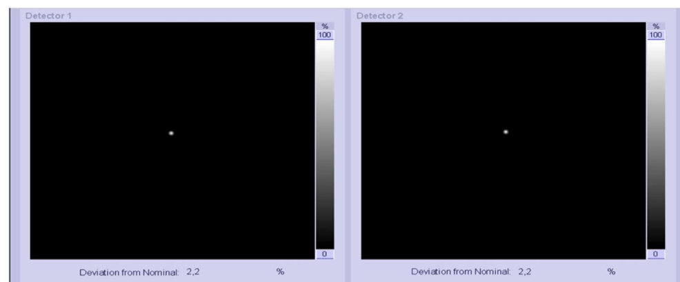
Figure 5. Planar images obtained from the system calibration with the ^{57}\text{Co} point source.
