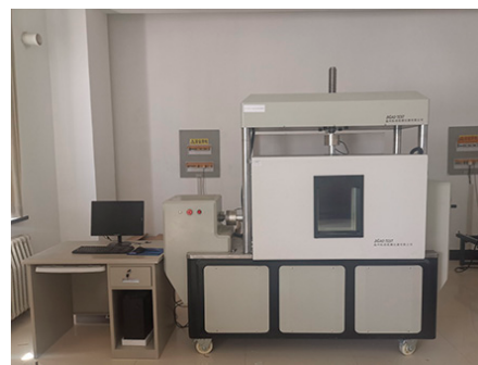
Figure 1. YT1200S direct shear pullout friction instrument for geosynthetics.
