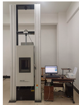
Figure 5. The electronic machine with controlled temperature.
