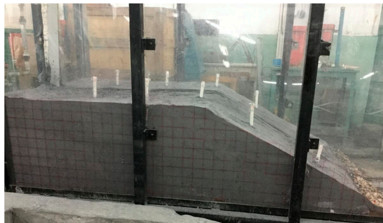
Figure 3. Pressure measuring pipes buried in the dam.
