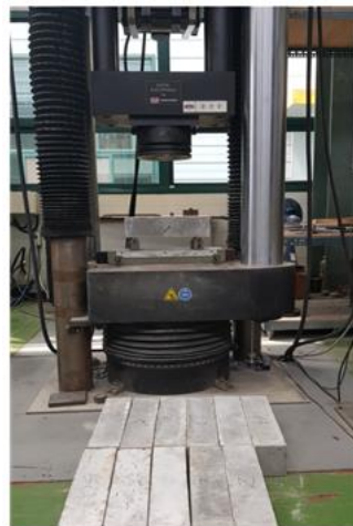
Figure 3. View of specimens and set-up for flexural performance test.
