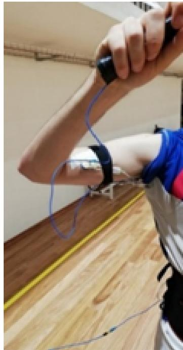
**Figure 4.** Electromyographic instrumentation of the athletes.
