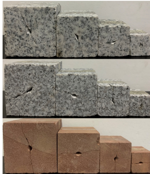
Figure 4. Images of point load damage in the three rock samples.
