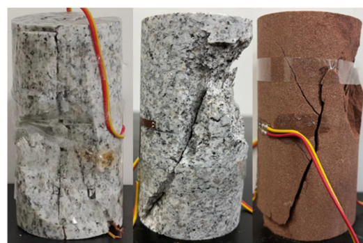
Figure 5. Images of uniaxial compression damage in the three rock samples.
