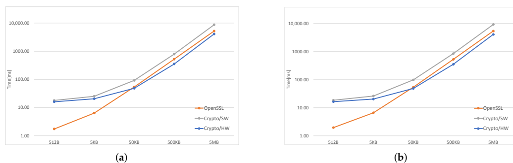
Figure 5. Time required to compute AES modes on increasing file sizes. (a) AES-ECB. (b) AES-CBC.
