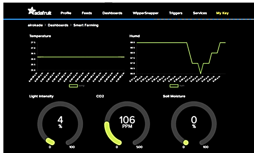
Figure 9. Sensor output on Adafruit IO Cloud IoT dashboard for Case 1.
