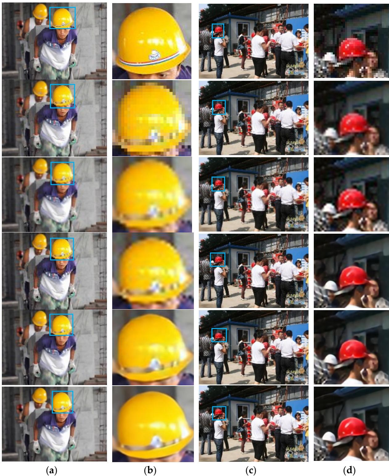
Figure 4. The comparison of the images produced by different SR method. From left to right, columns (a,c) indicate the complete images, columns (b,d) indicate the zoom-in regions defined by the blue bounding boxes. From the first row to the last row: original high-resolution image, images achieved via nearest neighbor interpolation, images achieved via bilinear interpolation, images achieved via bicubic interpolation, images achieved via DRN, images achieved via the proposed SR module.
