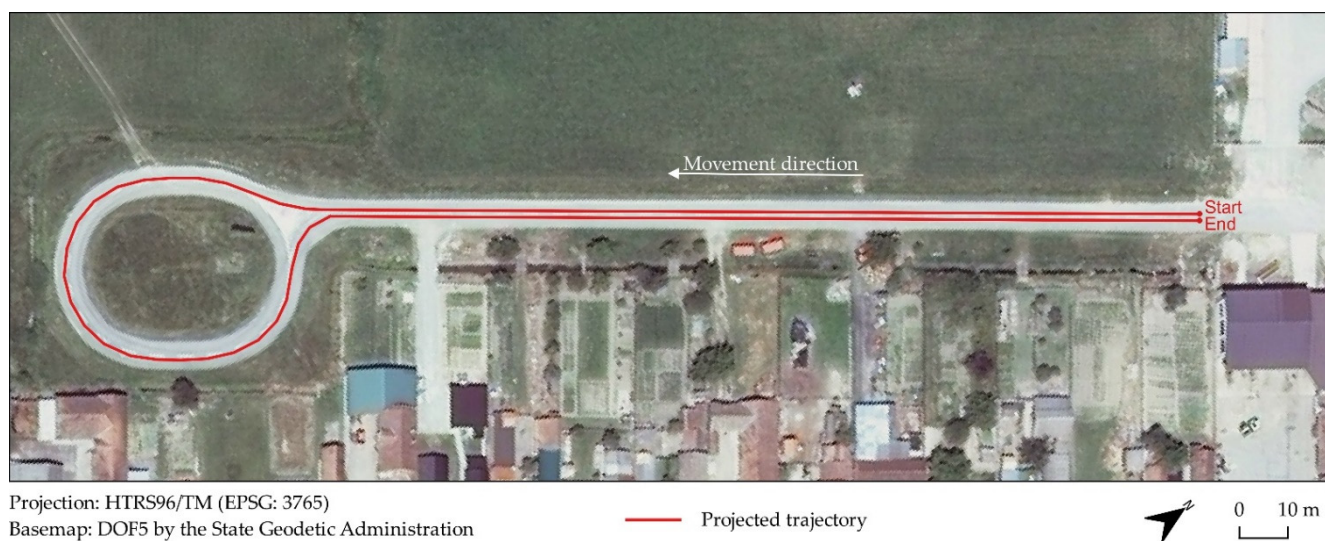
Figure 1. Study area and the trajectory for the accuracy assessment of GNSS RTK corrections.
