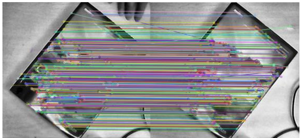
Figure 10. The improved ORB algorithm is used to extract feature matching images under overexposure conditions.
