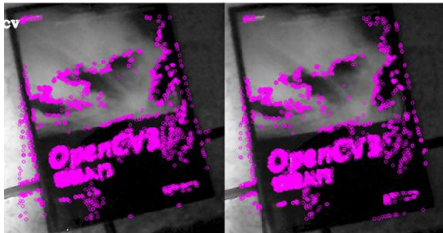
Figure 14. Feature points extracted by the improved ORB algorithm under underexposure conditions.
