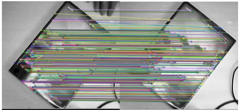
Figure 8. Feature matching image extracted by the traditional ORB algorithm under overexposure conditions.
