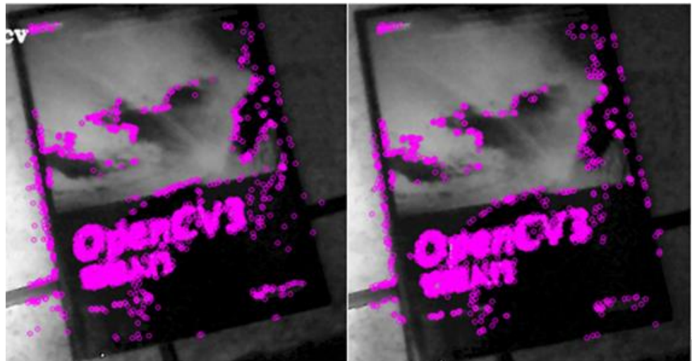
Figure 12. Feature points extracted by the traditional ORB algorithm under underexposed conditions.
