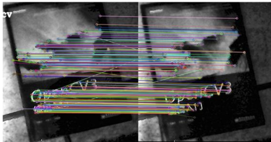
Figure 15. The improved ORB algorithm is used to extract feature matching images under underexposure conditions.
