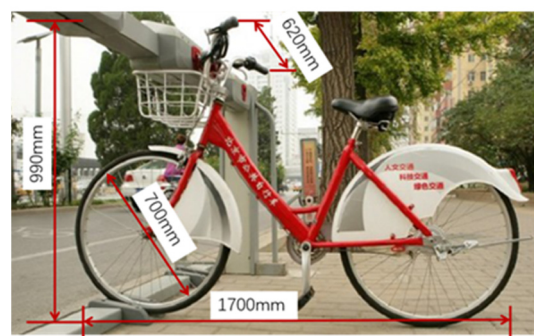
Figure 5. Dimensions of the typical bicycle.
