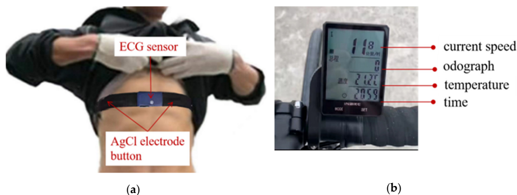
Figure 6. Main apparatus used in the field experiment. (a) BodyMon KF-2; (b) speedometer.
