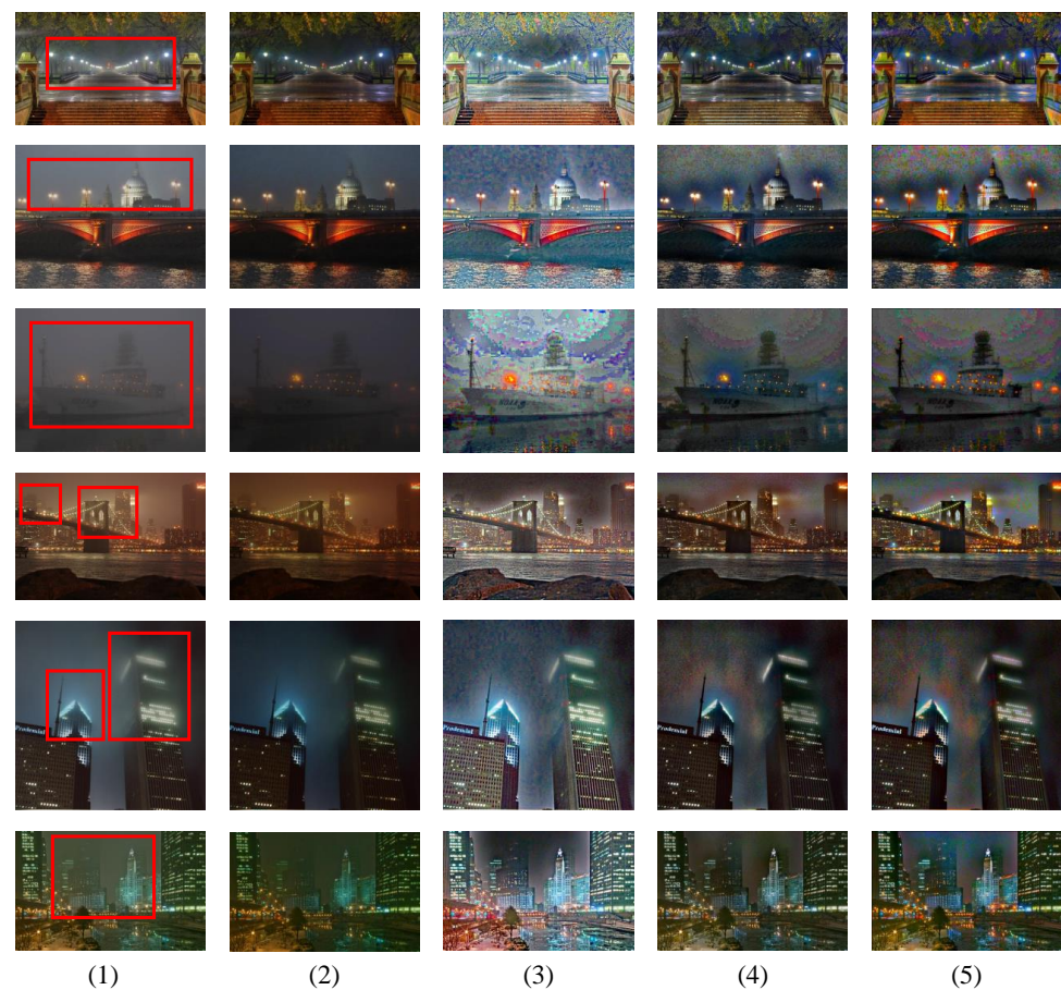
Figure 5. The objective experimental results. The defogging effect can be clearly seen at the red box (1) Nighttime hazy image. (2) DCP [14]. (3) NDIM [25]. (4) OSFD [35]. (5) OURS.
