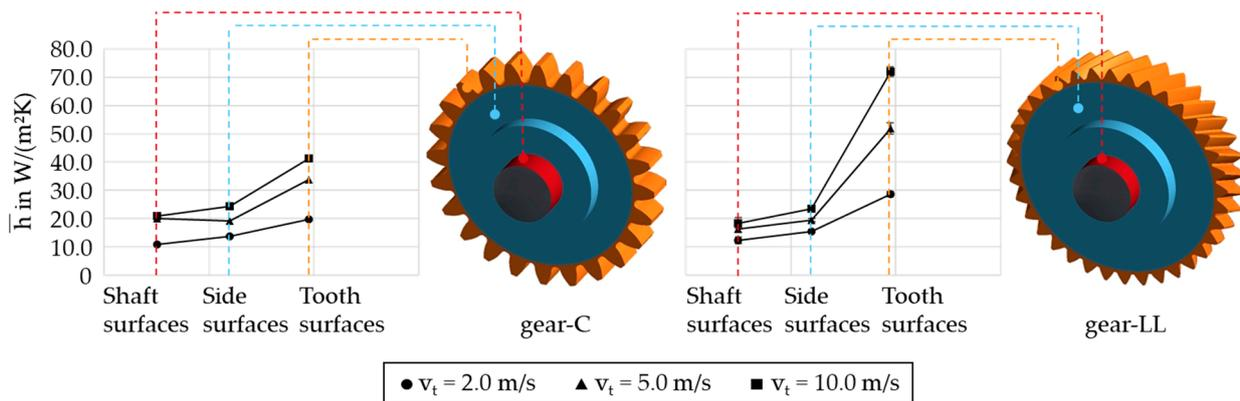
**Figure 10.** Surface-averaged HTC  $h$  for shaft, side, and tooth surfaces for the wheel of gear-C and gear-LL for circumferential speeds  $v_t = \{2.0; 5.0; 10.0\}$  m/s.
