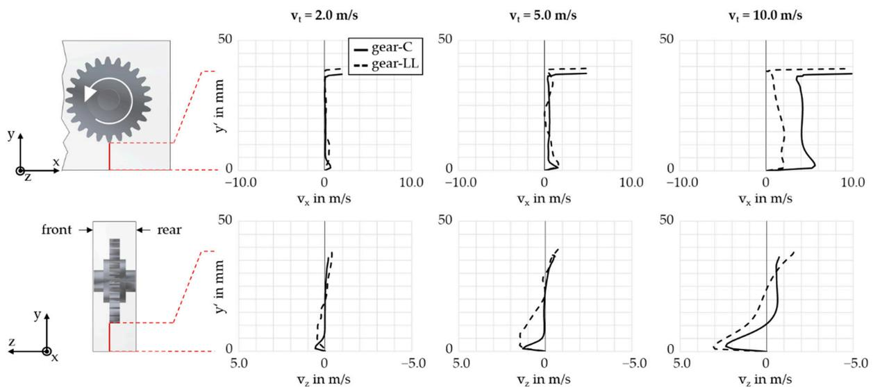
**Figure 6.** Flow velocities  $v_x$  and  $v_y$  below the wheel of gear-C and gear-LL for  $v_t = \{2.0; 5.0; 10.0\}$  m/s.
