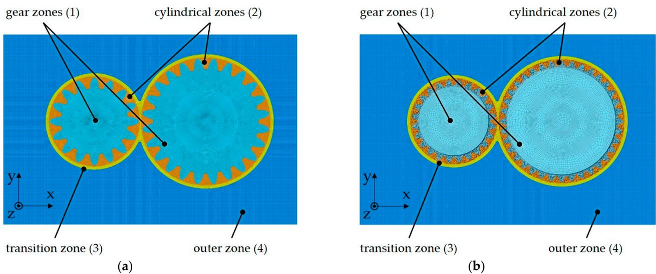
Figure 3. Front view on the mesh model Mesh<sub>gear-C</sub> (a) and Mesh<sub>gear-LL</sub> (b).
