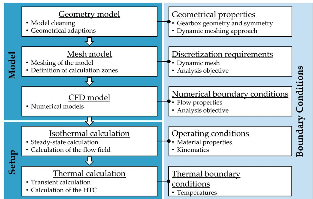
**Figure 4.** Simulation methodology for the thermal CFD simulations of the gearbox.
