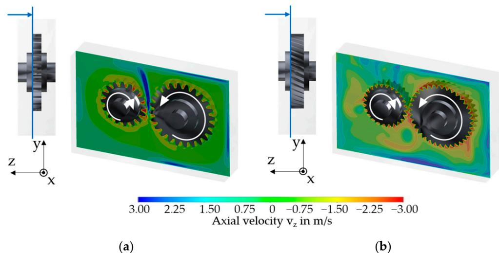
**Figure 8.** Axial flow velocity (z-direction) on a plane congruent to the side surface for gear-C (a) and for gear-LL (b) at circumferential speed  $v_t = 10.0$  m/s.
