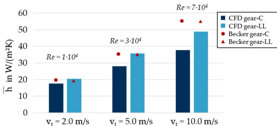
**Figure 11.** Surface-averaged HTC  $\bar{h}$  for gear-C and gear-LL for circumferential speeds  $v_t = \{2.0; 5.0; 10.0\}$  m/s in comparison to HTC based on Nusselt correlation according to Becker [15].
