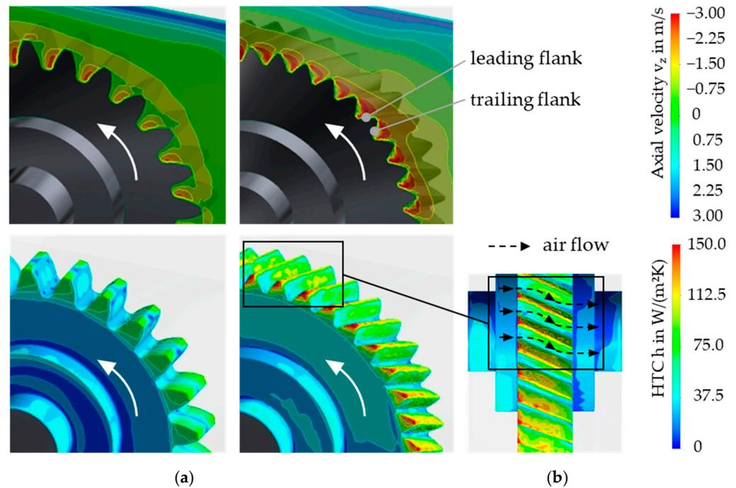
**Figure 9.** Detailed view on axial flow velocity ( $z$ -direction) and HTC between gear surface and air for the wheels of gear-C (a) and gear-LL (b) for  $v_t = 10.0$  m/s.
