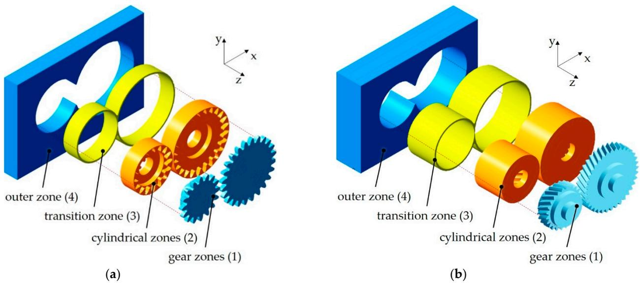
Figure 2. Modular structure of the geometry model for gear-C (a) and gear-LL (b).
