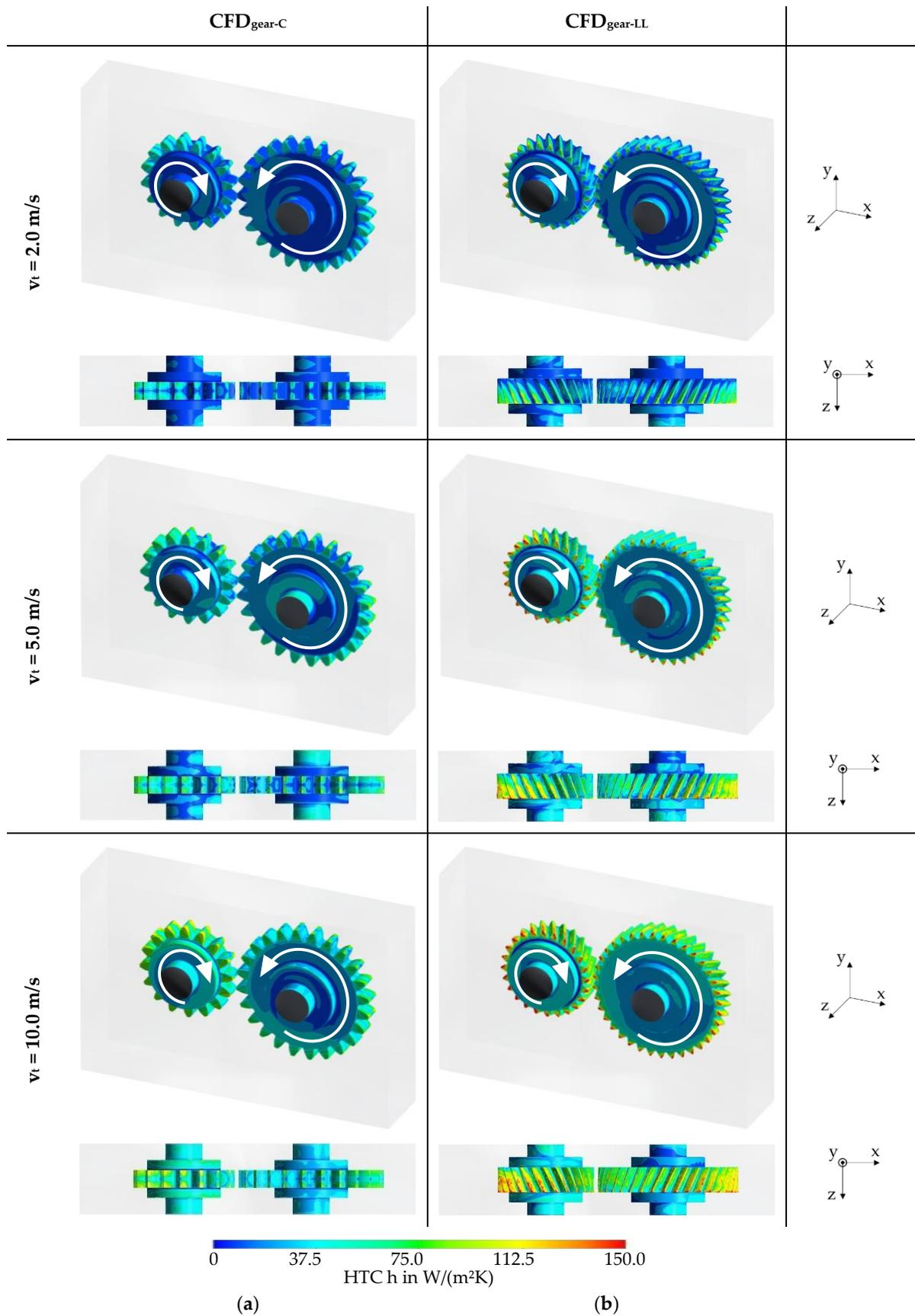
**Figure 7.** Heat transfer coefficient  $h$  between the gear surfaces and air for  $v_t = \{2.0; 5.0; 10.0\}$  m/s in 3D and top view for gear-C (a) and for gear-LL (b).
