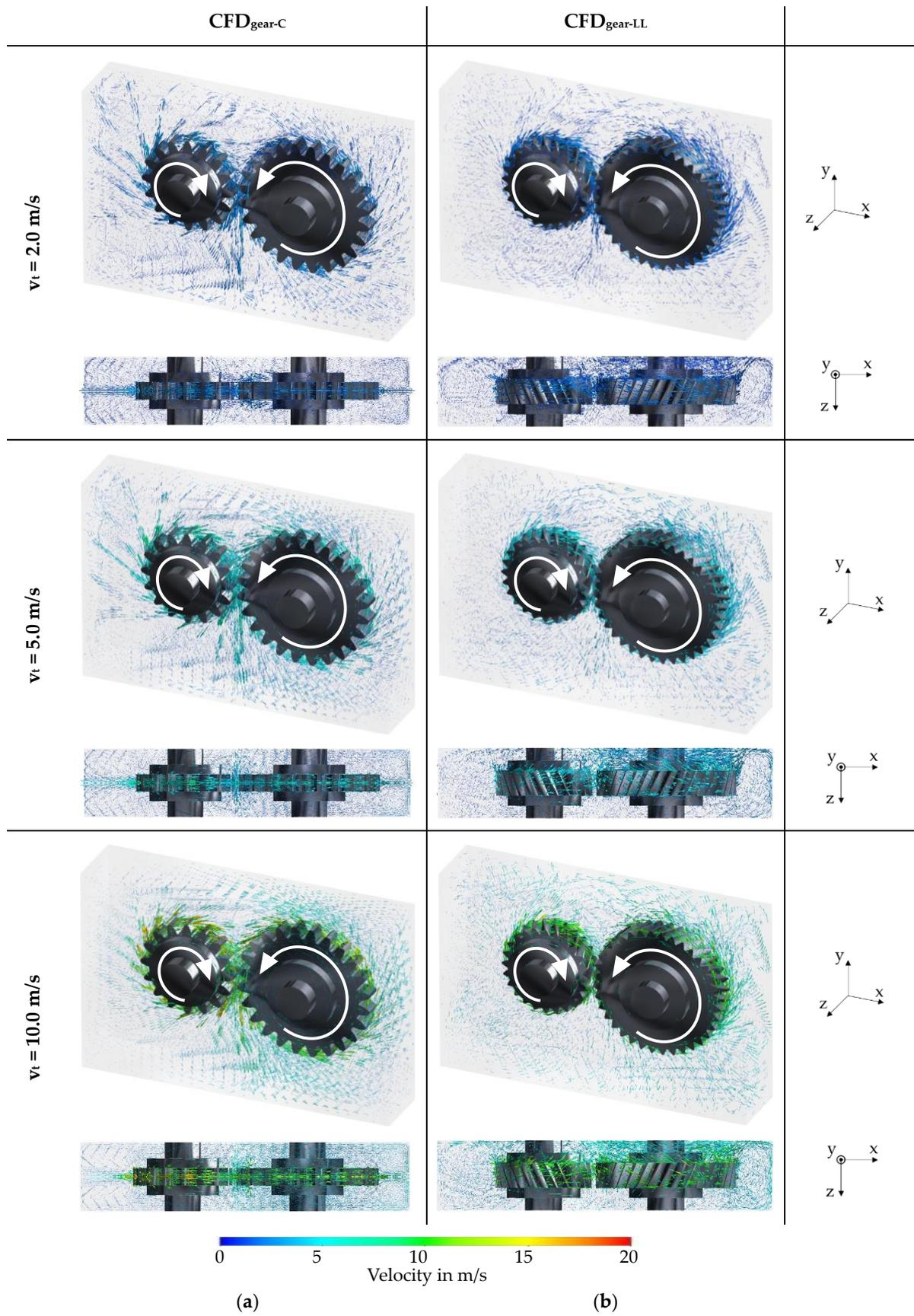
**Figure 5.** Isothermal flow fields in 3D view and top view for  $v_t = \{2.0; 5.0; 10.0\}$  m/s based on a steady-state calculation for gear-C (a) and gear-LL (b).
