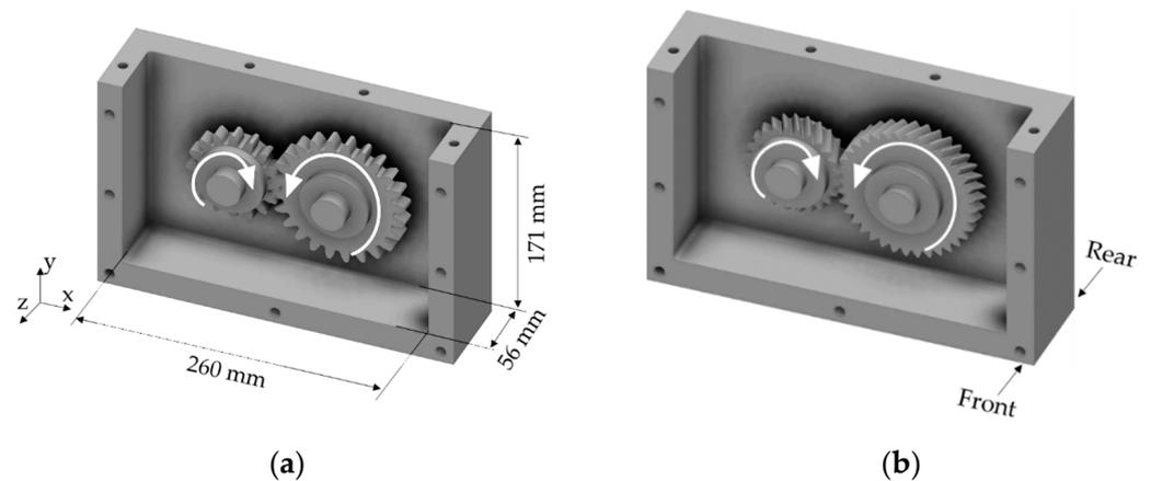
Figure 1. Considered test gearbox with gear-C (a) and gear-LL (b).
