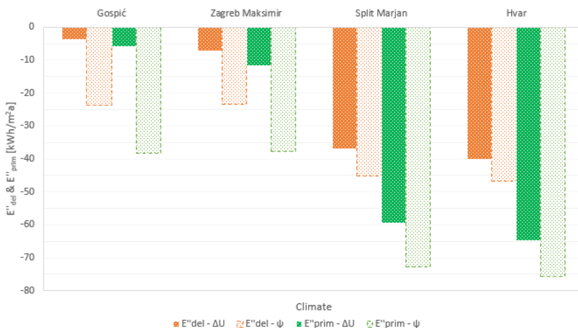
Figure 12. Delivered and primary energy use depending on the thermal bridge consideration approach.
