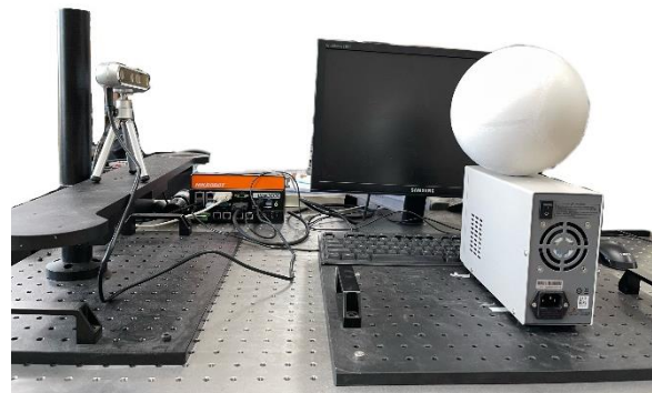
Figure 15. 3D reconstruction experiment using Intel Realsense D455.
