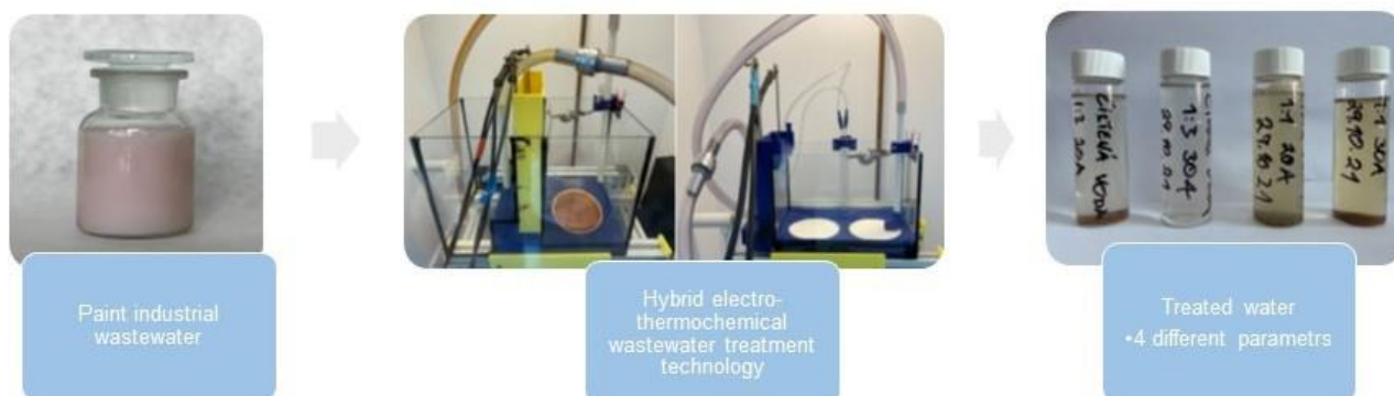
Figure 5. The hybrid electro-thermochemical wastewater treatment technology [6].
