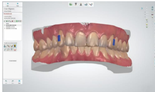
Figure 2. A 3Shape software used in this example to design a maxillary clear aligner.
