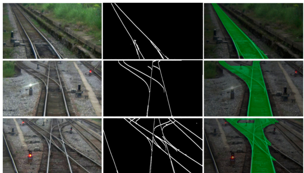
Figure 16. Multiple turnout track lines and track region extraction.
