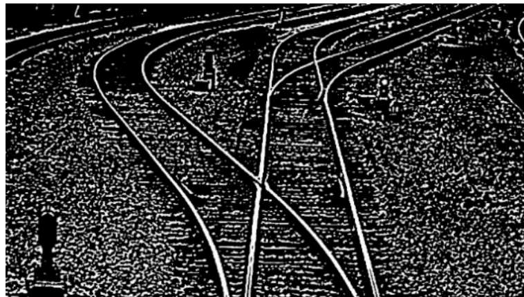
Figure 5. The result after adaptive threshold segmentation.
