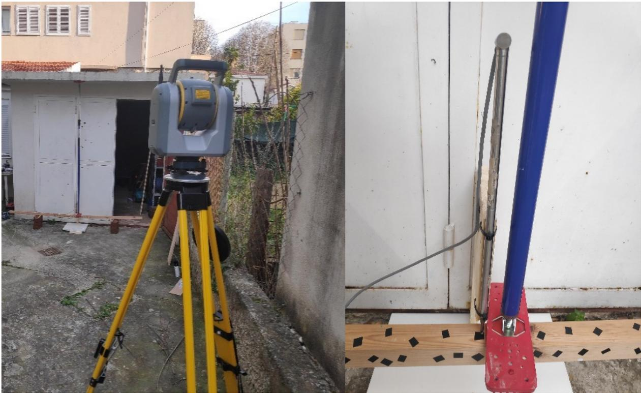
**Figure 3.** Test field (left) and test configuration (right) representing the wooden beam and LVDT (Source: Own compilation).
