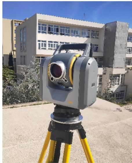
**Figure 1.** Trimble multi station SX10 (Source: Own compilation).
