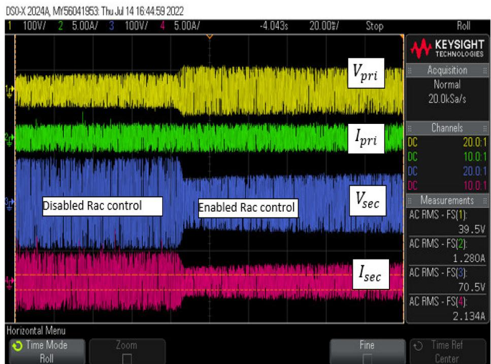
Figure 24. Transmitter/receiver coil current/voltage at  $V_o = 40\text{ V}$  with  $R_{dc} = 150\ \Omega$  connected when rectifier  $R_{ac} = 38\ \Omega$  feedback control is disabled vs. enabled.
