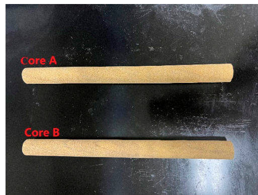
Figure 3. Physical picture of cores. Core A-300mD, Core B-600mD.
