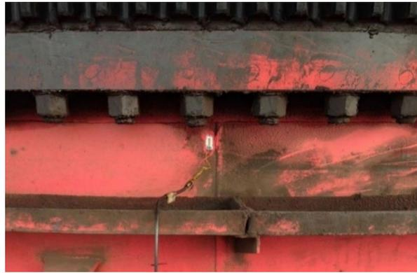
**Figure 11.** The actual location and method of laying the strain gauges.
