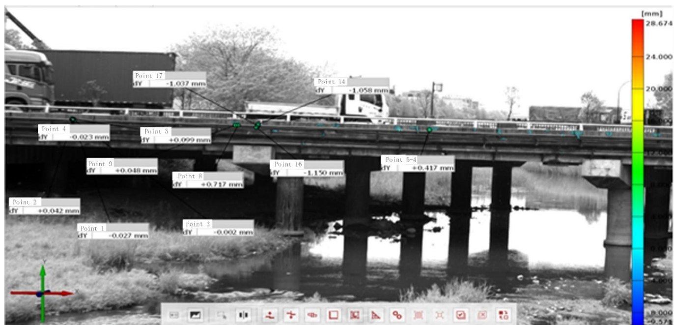
Figure 8. Interface of the monitoring system.
