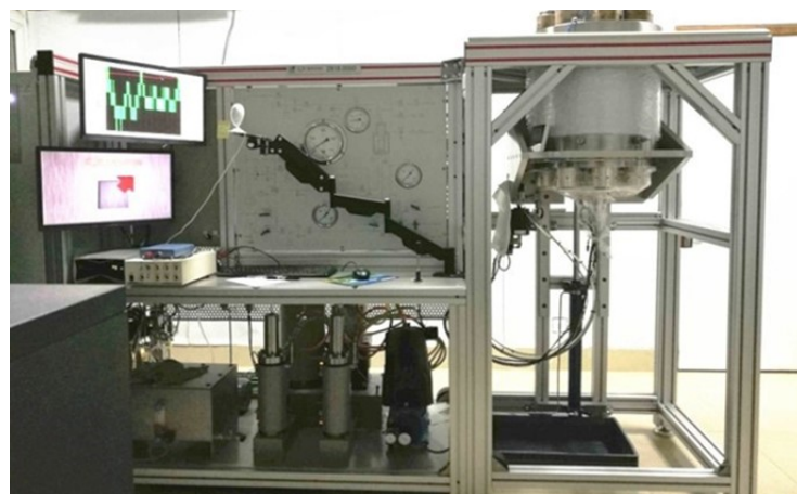
Figure 1. Servo-controlled rock triaxial testing system.
