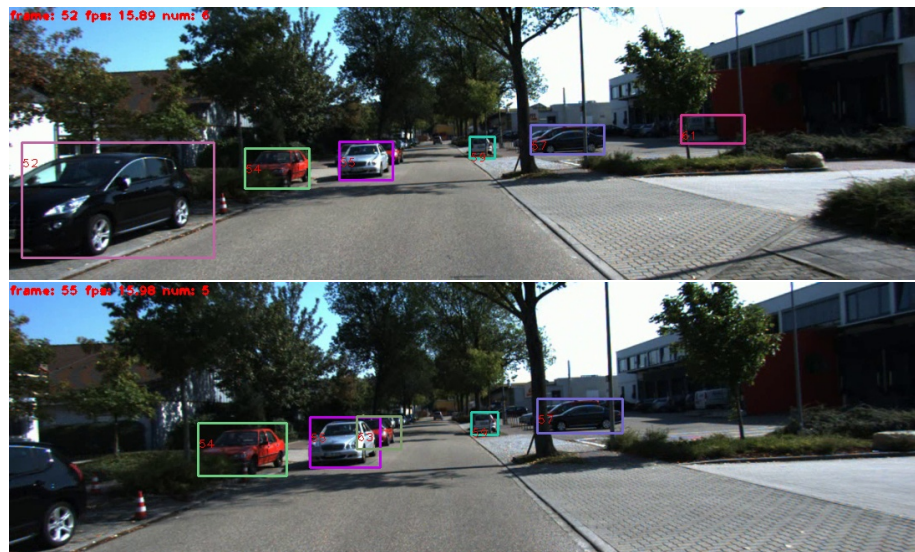
Figure 4. Qualitative results of our visual-based tracker on KITTI. The color of each bounding box indicates the target identity. The number of frames, fps and tracked objects is shown in the upper left corner of each image.
