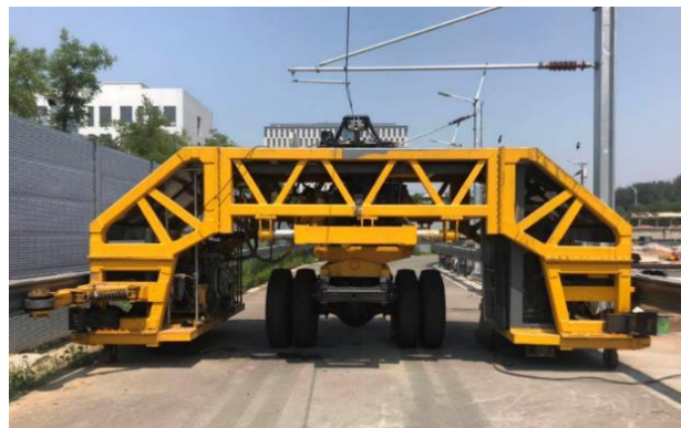
Figure 4. Full-scale accelerated loading test system.
