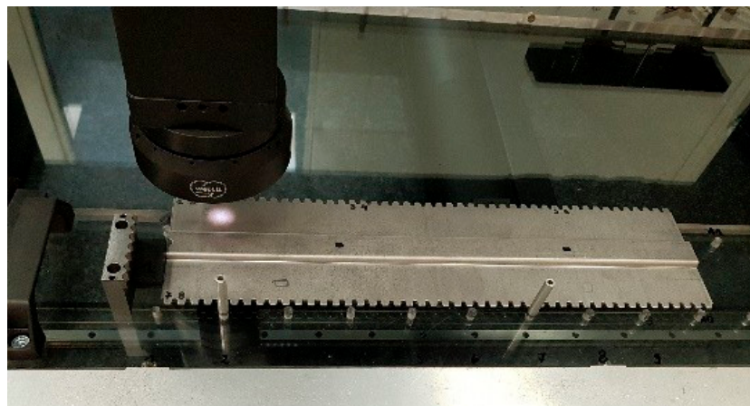
Figure 7. Measurement of the blank with the Multisensory Measuring Machine Werth Scope Check (blank placed on a glass plate) (own study).
