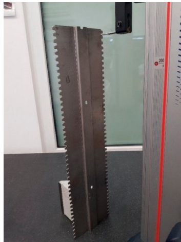
Figure 5. Measurement of the pattern with the LH-600 height gauge (the pattern is placed on the plate and fixed with a magnetic prism) (own study).
