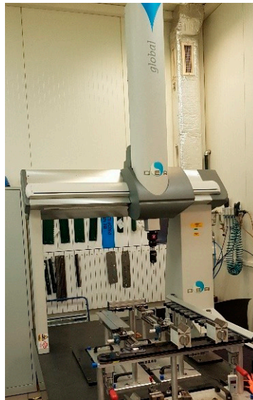
Figure 6. Measurement of the pattern with the DEA Global Coordinate Measuring Machine (the standard is mounted on a tripod and fixed with handles).
