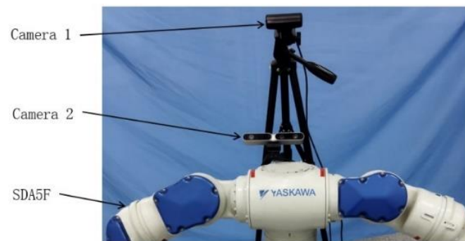
Figure 6. Setup of the two cameras in the dual-arm hand–eye robot system.
