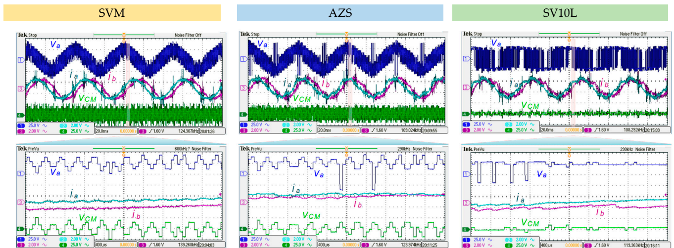
Figure 10. Experimental results of phase voltage, two of the line currents, and the CMV waveforms for the analyzed PWM schemes.
