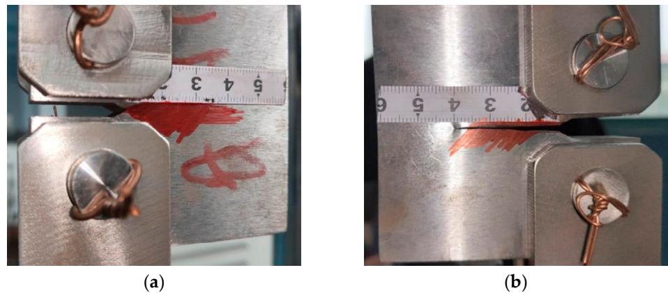
Figure 4. Fatigue crack propagation process. (a) Crack propagation initial stage; (b) Crack propagation close to fracture.
