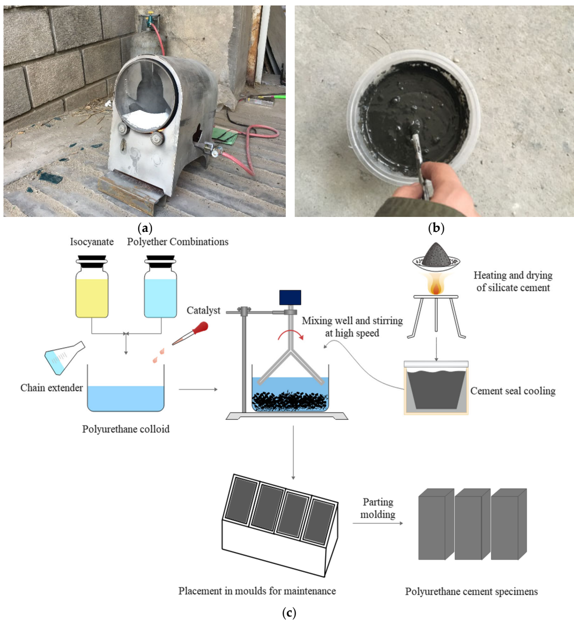
Figure 12. The preparation process of polyurethane cement: (a) stir frying cement; (b) stirring polyurethane cement; (c) preparation process flow chart.
