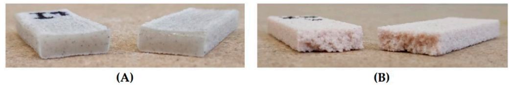
Figure 11. Example of fractured specimens. (A) Horizontally built specimen, with 0% sand, displaying a smooth fracture surface. (B) A similar specimen built with 60% sand, displaying a granular and irregular type of fracture surface.
