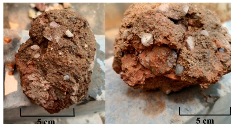
Figure 6. Clay-cobble mixture collected at the ring 145 at the Beijing south-to-north water diversion auxiliary project.
