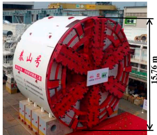
Figure 8. The used shield machine at the Jinan Huanghe River Crossing tunnel.
