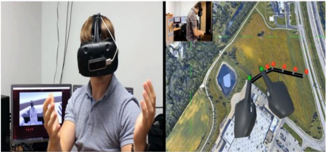
Figure 13. Use of HTC VIVE head-mounted display with Leap Motion optical tracking [43].
