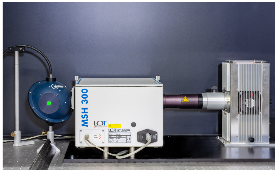
Figure 4. Image representation of the monochromator setup used in this work.
